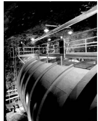
Fig. 6.18 The detector of the chlorine experiment of R. Davis for the measurement of solar neutrinos. The detector is installed at a depth of 1400 m in the Homestake Mine in South Dakota. It is filled with 380 000 liters of perchlorethylene {11}
