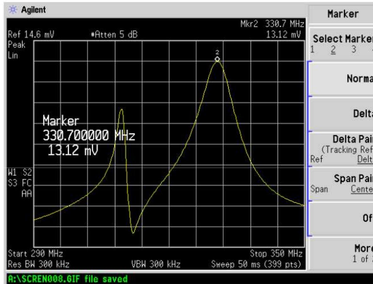
**Deuterium** Scan of the deuterium resonator between 290 and 350 MHz. The vertical linear scale shows the PU voltage of the fixed coil placed near the grounded end of the uncoupled D rod (see Fig. 3 and 8). The upper peak at 330.7 MHz corresponds to the required counter mode, the lower one to the common mode.
