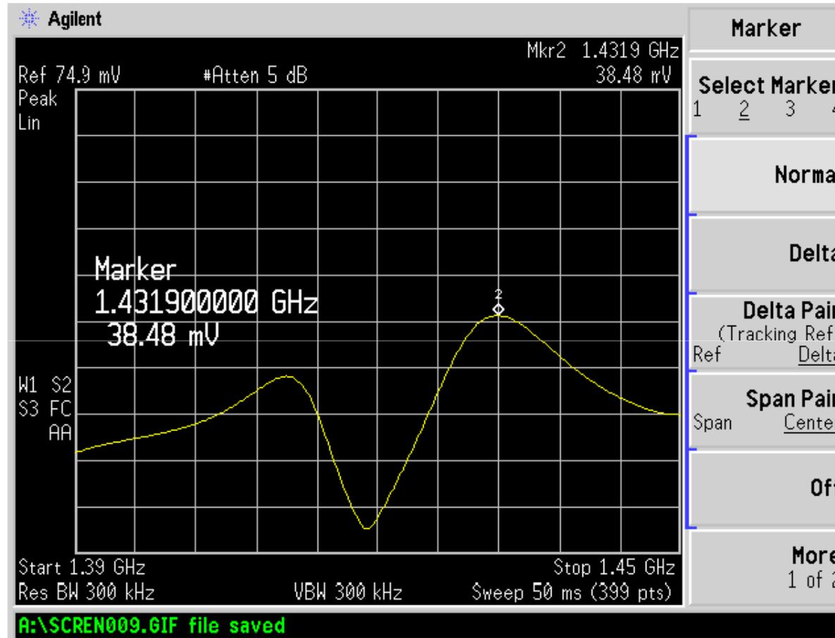
**Hydrogen** Scan of the hydrogen resonator between 1.39 and 1.45 GHz. The vertical linear scale shows the PU voltage of the fixed coil placed near the grounded end of the uncoupled H rod (see Fig. 3 and 8). The upper peak at 1.432 GHz corresponds to the required counter mode, the lower one to the common mode.
