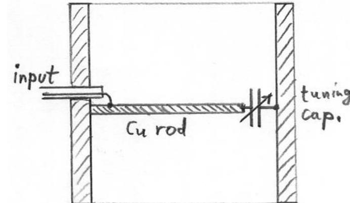
Conducting rod of length  $a$  grounded at the left corner. The voltage and current distribution of a fictitious rod of length  $\lambda/4 = a + \Delta$  is shown. The difference  $\Delta$  is accounted for by a load capacity between the end of the rod and the ground to the right.
