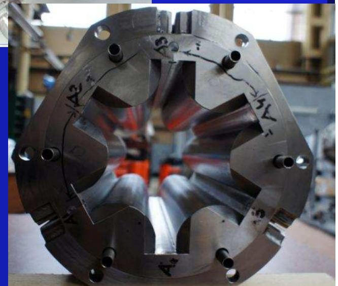
Sextupole corrector prototype (for SIS100 & NICA booster) at assembly
