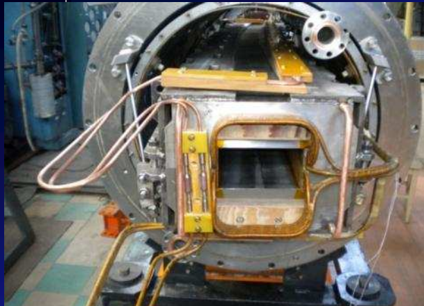
Booster dipole at cryo-test (9.7kA) & magnetic measurements
