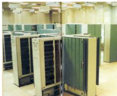
10-processing complex «Elbrus» 120 million operations per second
