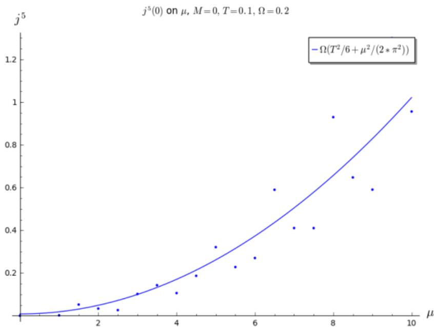
FIG. 10: The axial current density at  $r = 0$  (given in the units of  $R^{-3}$ ) as a function of  $\mu$  (given in the units of  $R^{-1}$ ) for the system of massless fermions rotating with the angular velocity  $\Omega = 0.2R^{-1}$ .
