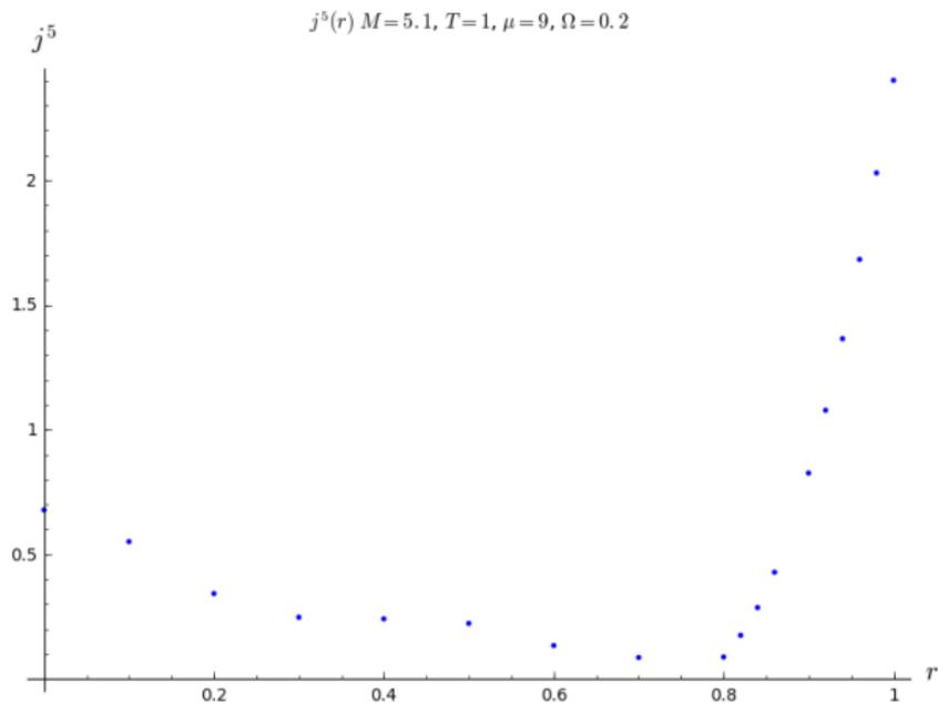
FIG. 6: The axial current density (given in the units of  $R^{-3}$ ) as a function of  $r$  (given in the units of  $R$ ) for the system of fermions with  $M = 5.1R^{-1}$  rotating with the angular velocity  $\Omega = 0.2R^{-1}$ . Temperature is taken equal to  $T = 1R^{-1}$ . The value of the chemical potential is  $\mu = 9R^{-1}$ .
