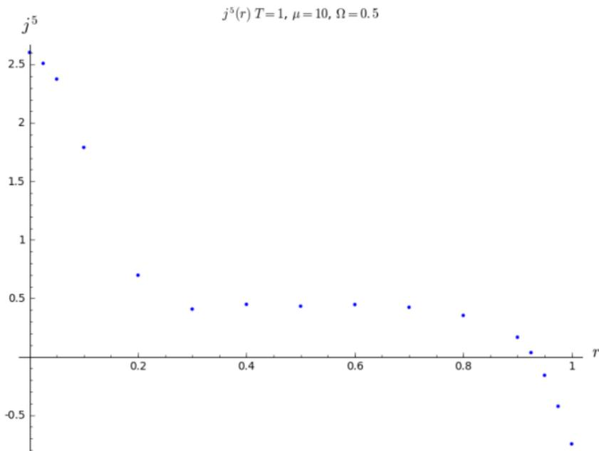
FIG. 4: Axial current density as a function of  $r$  (given in the units of  $R$ ) for the system of massless fermions rotating with the angular velocity  $\Omega = 0.5/R$ . Temperature is taken equal to  $T = 1/R$ . The value of chemical potential is  $\mu = 10/R$ .
