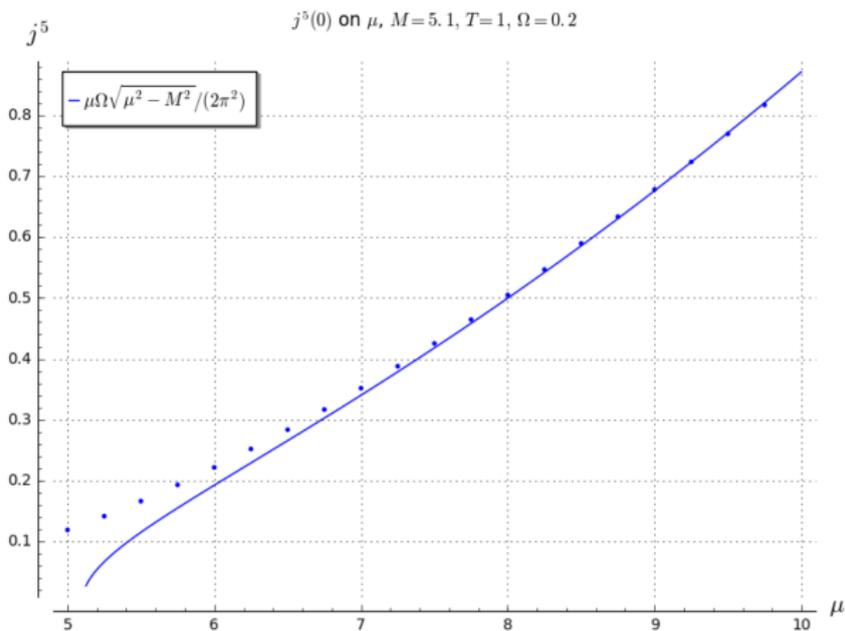
FIG. 7: Axial current density at  $r = 0$  as a function of  $\mu$  (given in the units of  $1/R$ ) for the system of fermions with mass  $M = 5.1/R$  rotating with the angular velocity  $\Omega = 0.2/R$ . Temperature is taken equal to  $T = 1/R$ .
