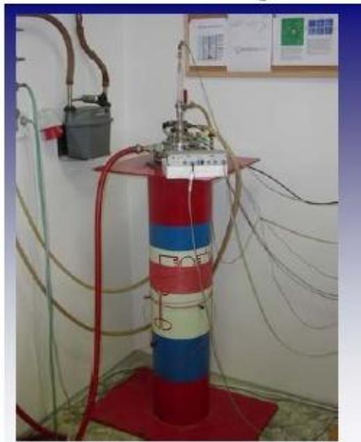
One of two noncommercial SQUID magnetometers used for investigation.
