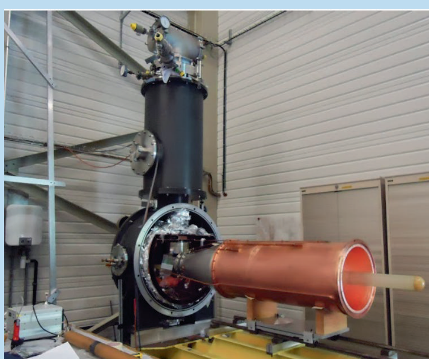
Fig. 2: Dilution refrigerator, microwave cavity and mixing chamber.
