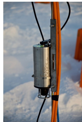
Underwater acoustic modem
