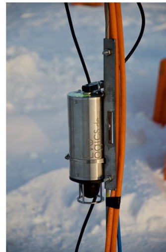
Underwater acoustic modem
