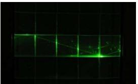
The **Raghavan Optical Lattice** (ROL), invented by the late Virginia Tech professor, Raju Ragahvan, divides a totally active volume into cubical cells that are read-out by total internal reflection. LENS was designed for solar neutrino detection and not optimized for reactor antineutrino detection.
