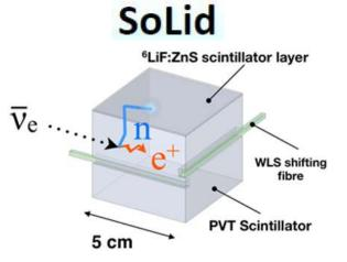
Optically isolated cubes, mated to <sup>6</sup>LiF:ZnS(Ag) sheets, are used to tag IBD. Light is read-out by wavelength shifting fibers in orthogonal directions. It has the spatial resolution of the ROL optimized for reactor antineutrino detection. The small cross-sectional area of the fibers limits the light collection, dilutes the energy resolution and lowers the efficiency.
