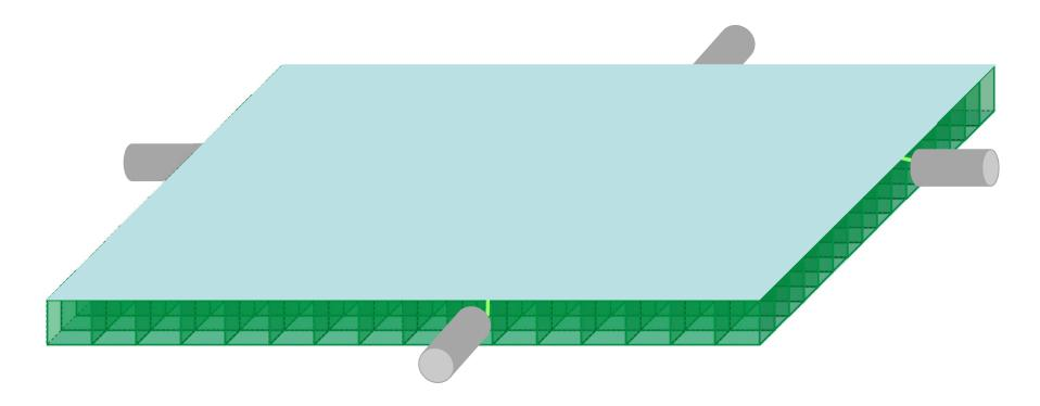
The light is transported to the detector's edge by total-internal-reflection and readout by PMTs.
