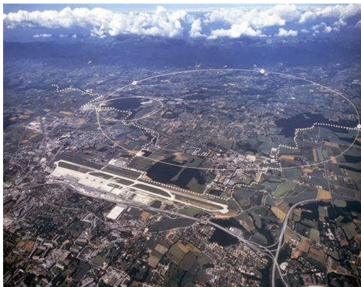
Aerial view of the CERN site just outside Geneva. The underground particle accelerators (with circumferences of 27 km and 7 km) allow scientists to look at tiny scales. Image © CERN .
