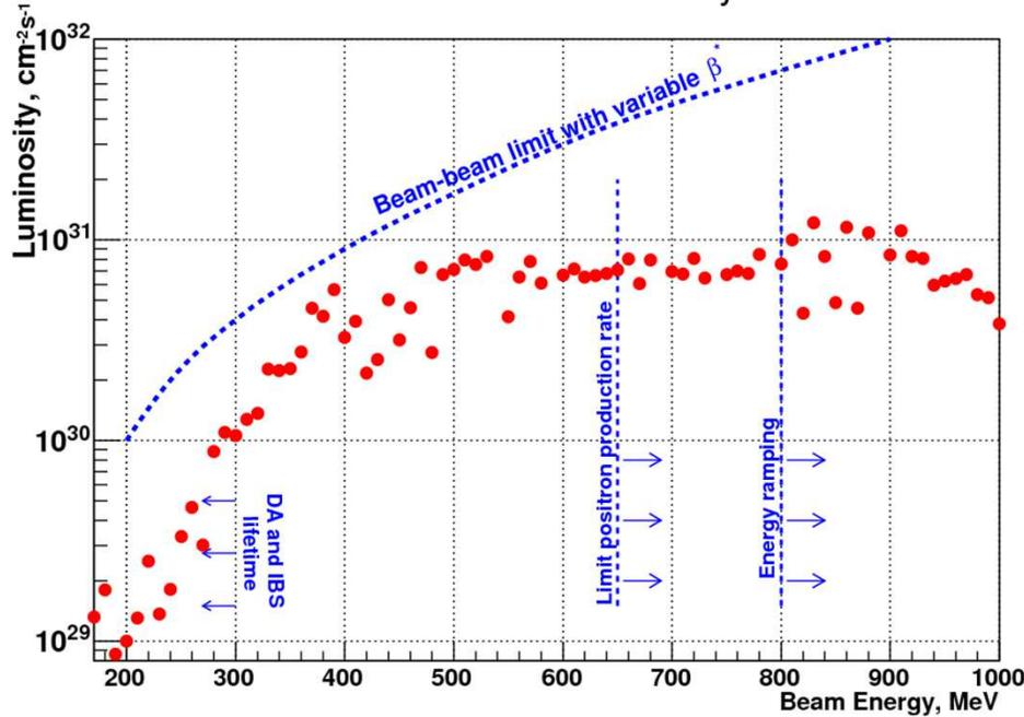
The maximum luminosity is  $2 \cdot 10^{31} \text{ cm}^{-2}\text{s}^{-1}$  at 1.7-1.8 GeV, falling much slower with decreasing energy than before the round beams
