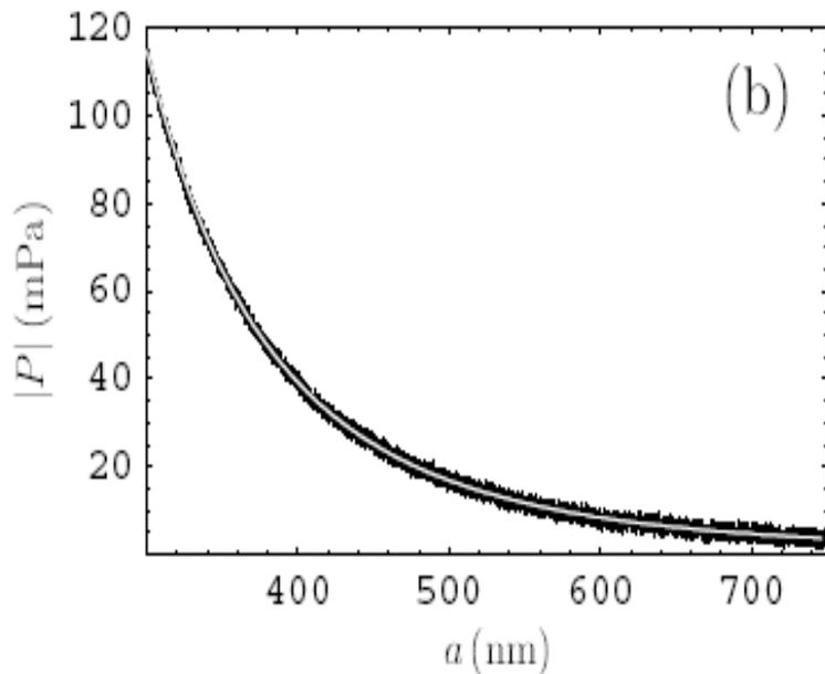
**Measurement data obtained using an AFM are shown as crosses with total experimental errors determined at a 67% confidence level.**
