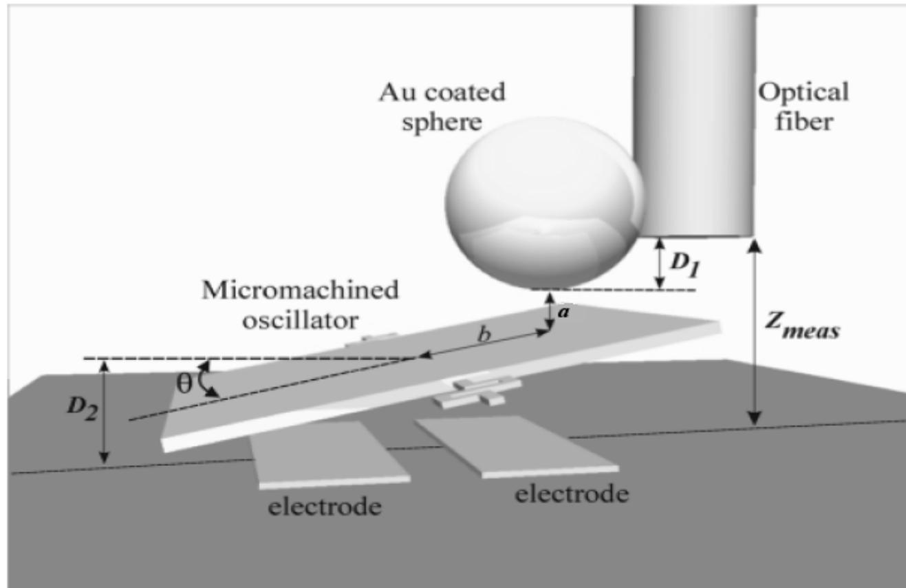
**Schematic setup with a micromachined oscillator**
