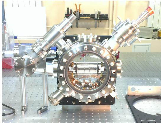
Рис. 1: Linear quadrupole Paul trap for simultaneous confinement of aluminum and magnesium ions
