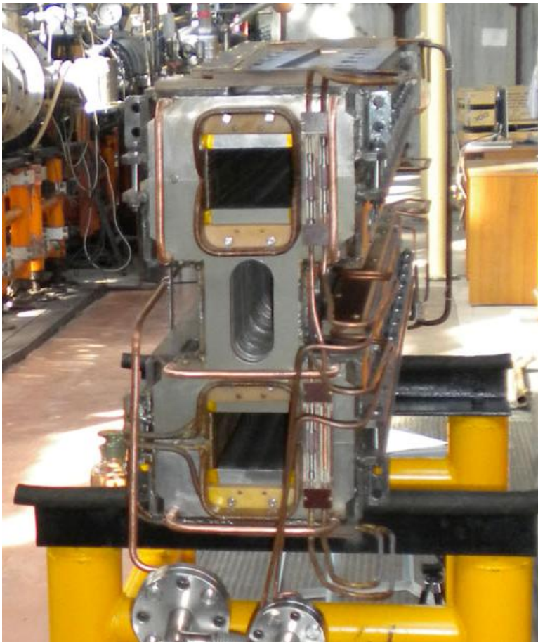
Test on vacuum tightness of the tubes for cooling the yoke
