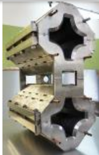
Booster dipole at cryo-test (9690A) and magnetic measurements
