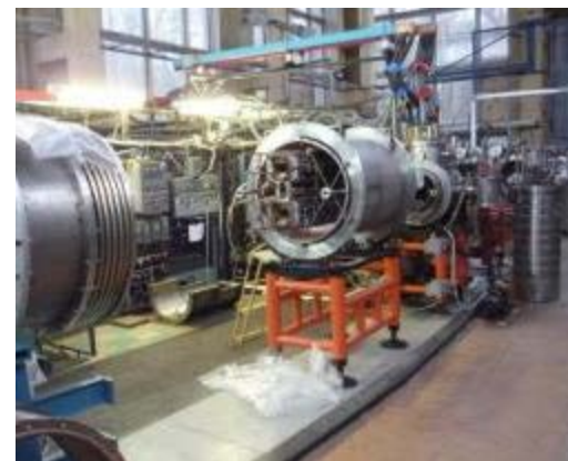
Sextupole corrector prototype (for SIS100 and NICA booster) at assembly
