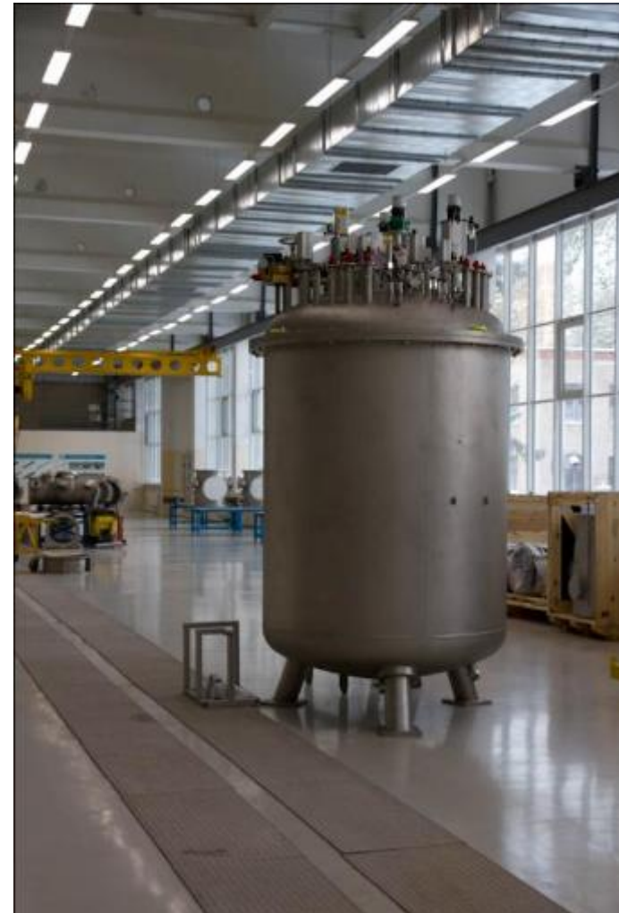
Satellite helium refrigerator in b.217. 59
