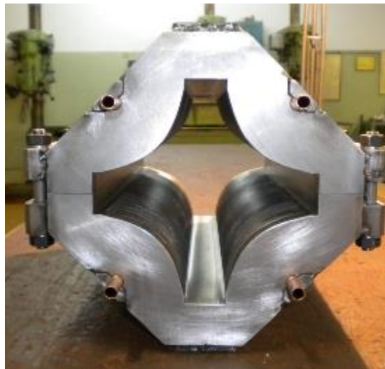
Quadrupole lense at assembly for test
