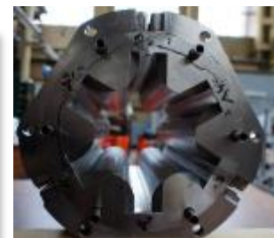
Sextupole corrector prototype (for SIS100 and NICA booster) at assembly
