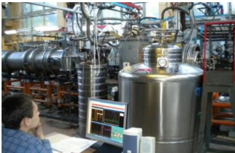
Cryogenic test-bench @ LHEP
