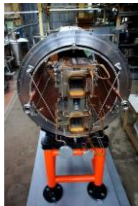
Twin aperture dipole magnet for Collider was tested June 2013 up to 11 kA
