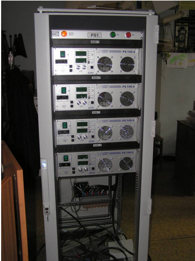
Kit of new power supplies (130 A) for Nuclotron correctors Collaboration with Slovakia
