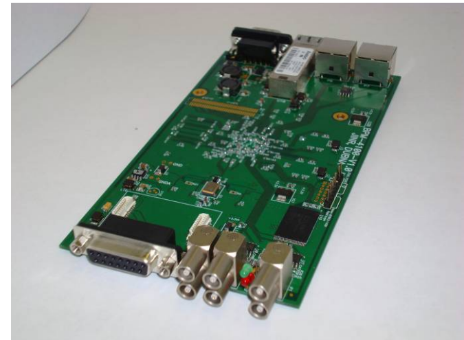
One of 30 chips (hi-tech) for automatic System for beam orbit measurement
