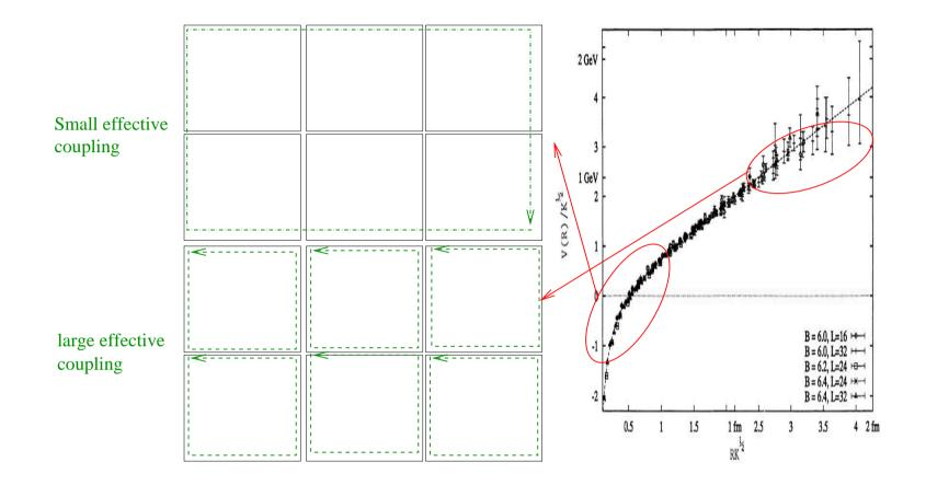
At large distances, such a loop ("the Wilson loop") depends on "area", ie the potential  $\propto r$  . At low distances, it depends on perimeter, so potential  $\propto r^{-1}$
