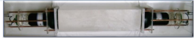
CsI(Tl) Crystal 8 \times 8 \times 30 \text{ cm}^3 (8.7 kg) 3" PMT (9269QA) : Quartz window, RbCs P.C. \sim 5 Photo-electrons/keV
