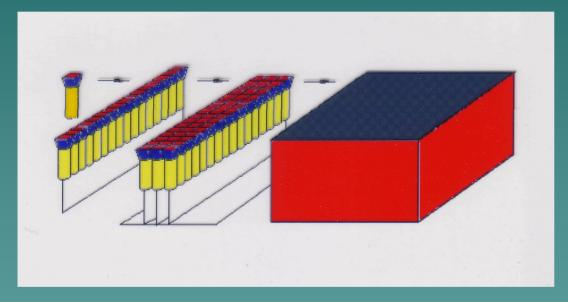
Photo receiver is consisted of 16 pixel rows and columns. Every pixel is a PM tube (Hamamatsu R1463, 13 mm diameter multialcali cathode) with a square window mirror light guide. 16 PM tubes (a row) has a common voltage supply and are controlled by one data acquisition unit. UV filter cover all pixel windows.
