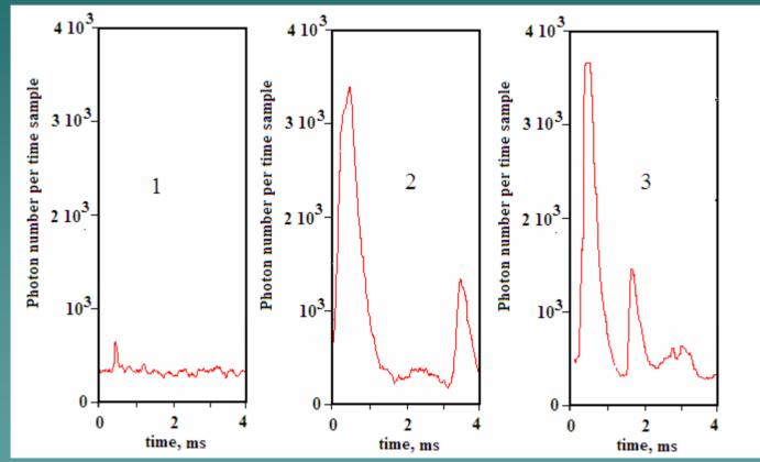
UV flashes registered by the "Tatiana" detector. Oscilloscope trace- 64 ms. UV energy in the atmosphere 0.1-1MJ.
