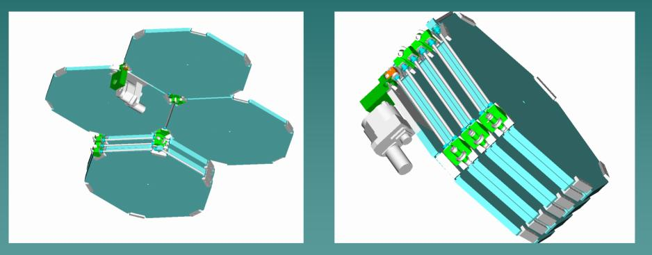
In this mechanism one electric motor moves the segments via axles and cardan joints.
