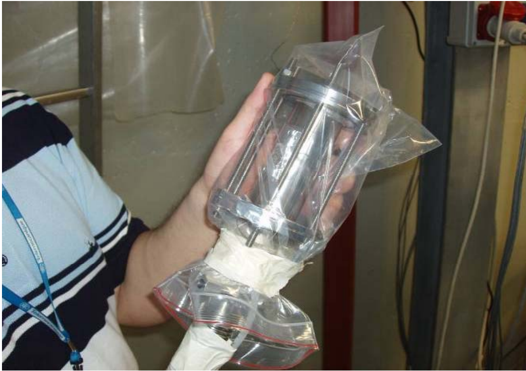
Fig.3. The Ti-SS transition sample wrapped with a plastic bag for the leak test measurements.
