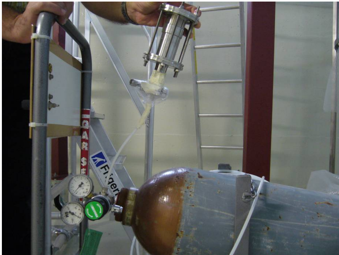
Fig.7. The sample connected to the helium bottle and filled with gaseous helium up to a pressure of about 6 bar
