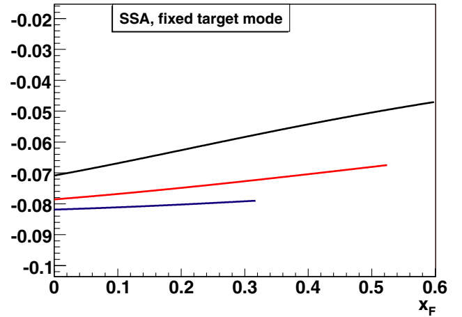
FIG. 6 (color online). SSA given by Eq. (20) versus x_F for the fixed target mode for three values of Q^2 : 16 \text{GeV}^2 (lower curve), 9 \text{GeV}^2 (middle curve), and 4 \text{GeV}^2 (upper curve).
