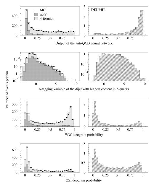
Fig. 5. Hq $\bar{q}$  channel: distributions of relevant analysis variables at the preselection level. The eight variables used to reduce the q $\bar{q}(\gamma)$  background are summarized by the output of the anti-QCD neural network. Data at  $\sqrt{s}=200$ –209 GeV (dots) are compared with Standard Model background expectations (left-hand side histograms) and with the expected distribution for a 114 GeV/ $c^2$  Higgs mass signal (right-hand side histogram).
