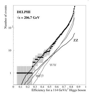
Fig. 4. Hq $\bar{q}$  channel: Expected Standard Model background rate at a centre-of-mass energy  $\sqrt{s} = 206.7$  GeV as a function of the efficiency for a 114 GeV/ $c^2$  Higgs mass signal when varying the cut on the neural network variable. The different background contributions are shown summed and separately. Dots stand for data.
