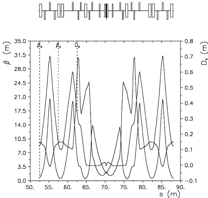
Fig. 2. Lattice functions in the wiggler quadrant (the wiggler is on).
