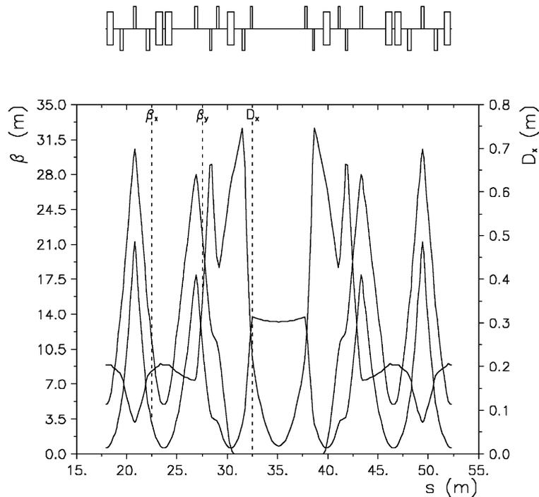
Fig. 1. Lattice functions in the matching cell and the straight section for the undulator.
