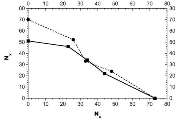
Fig. 3. The dynamic aperture, expressed as a multiple of the standard deviation with the wiggler off (solid line) and on (dotted line).
