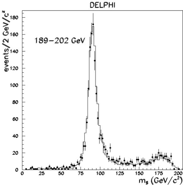
Fig. 4. Photon recoil mass spectrum for the  $\gamma gg$  candidates (points) and the expected background (histogram).
