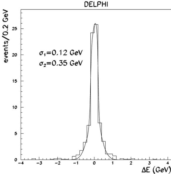
Fig. 2. The energy resolution  $\Delta E$  for the photons of the  $\gamma\gamma\gamma$  candidates in the QED  $e^+e^- \rightarrow \gamma\gamma(\gamma)$  simulated sample. The photon energy was obtained using (5). A fit with two Gaussians gave two resolution components  $\sigma_1 = 0.12$  GeV and  $\sigma_2 = 0.35$  GeV with approximately equal frequencies.
