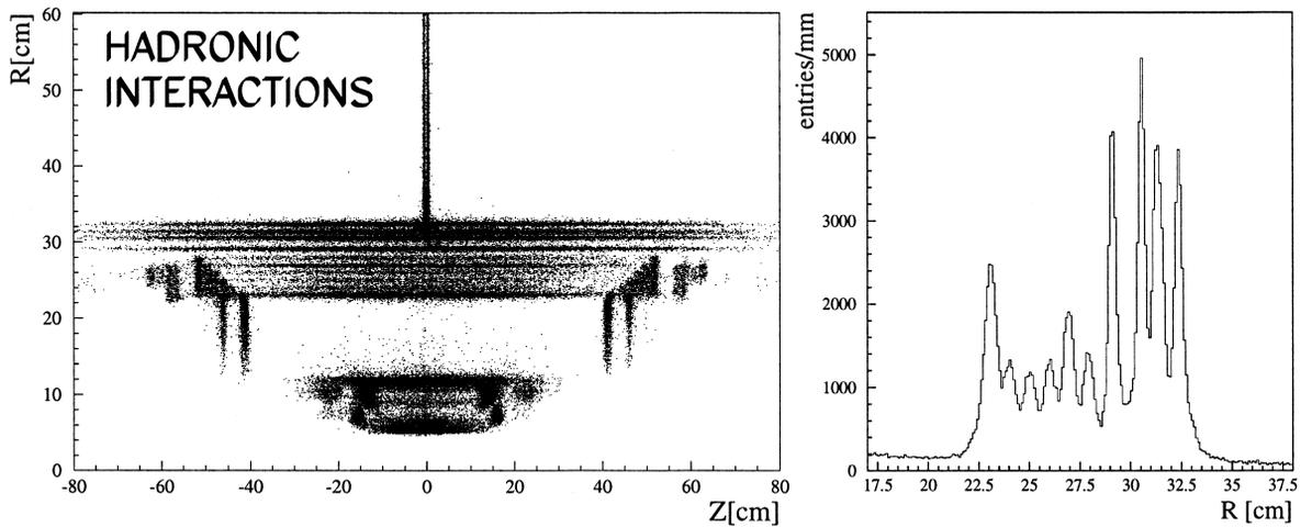
Fig. 1. Reconstructed hadronic interactions in the material of the DELPHI detector, used for the determination of the correction factor for the VD track efficiency. Left:  $Rz$  view; Right: Radial projection.
