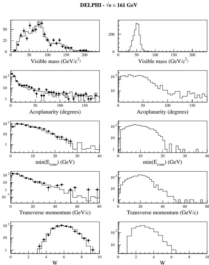
**Fig. 6.**  $h\nu\bar{\nu}$  channel, probabilistic analysis: distributions of some analysis variables as described in the text. Plots on the left show a comparison between 161 GeV data and simulated background events (*solid line*) normalised to the experimental luminosity. Plots on the right show the (unnormalised) expected distributions for a Higgs boson of  $60 \text{ GeV}/c^2$
