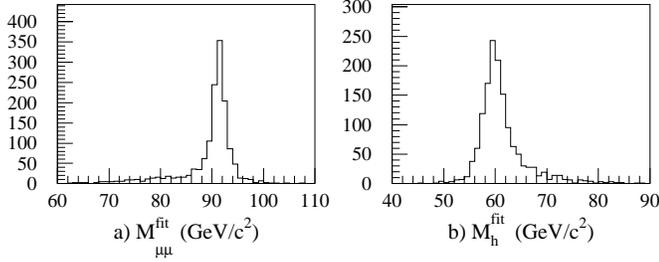
**Fig. 3.**  $h\mu^+\mu^-$  channel: distributions of **a** the Z mass and of **b** the Higgs boson mass at the end of the analysis for simulated  $h\mu^+\mu^-$  events with  $m_h = 60$  GeV/ $c^2$  at 161 GeV
