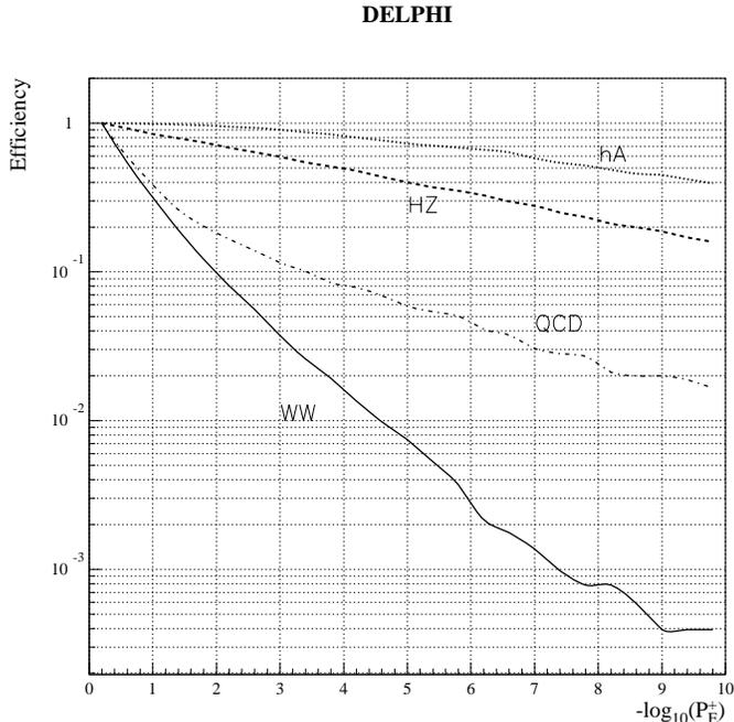
**Fig. 1.** Performance of the probabilistic b-tagging: efficiency of the b-tagging requirement based on a minimal value of  $-\log_{10}(P_E^+)$ , as a function of this value. The efficiency is within the acceptance of the vertex detector. Curves are shown for simulated hadronic 4-jet events from WW pairs and  $q\bar{q}(\gamma)$  background events (labelled ‘QCD’), and from hZ and hA signal events. Centre-of-mass energies of 161 and 172 GeV give similar results and have been combined
