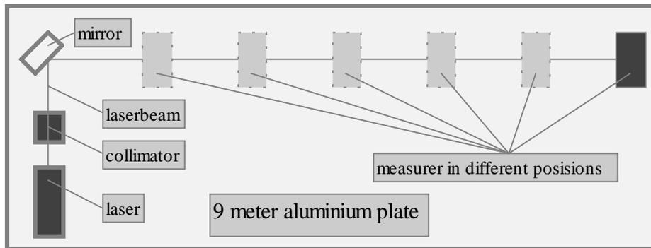
Figure 3. The scheme of the module measurer prototype.
