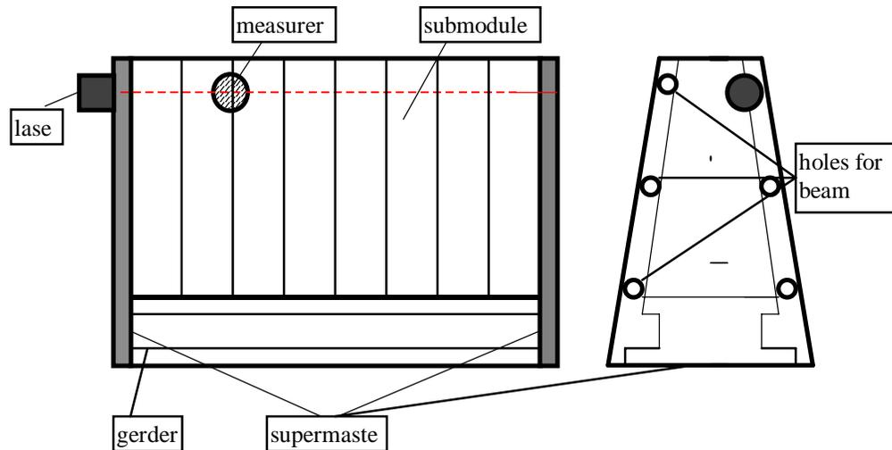
Figure 1. The scheme of the module size measurement.
