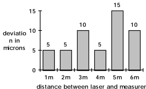
Figure 4. The maximum deviations at different laser-measurer distances.
