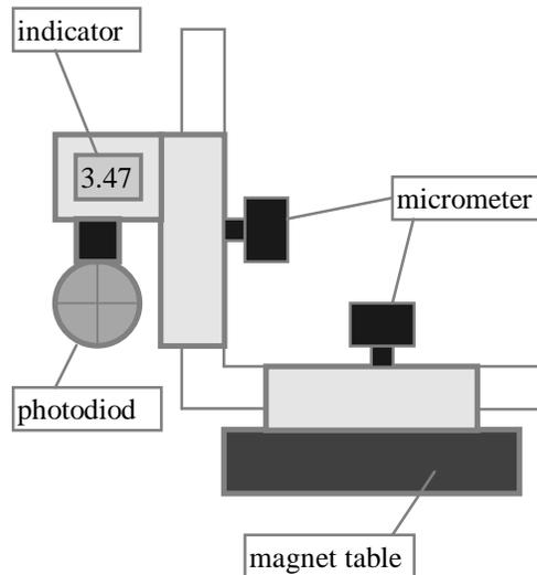
Figure 2. The device for beam-surface distance measurement.
