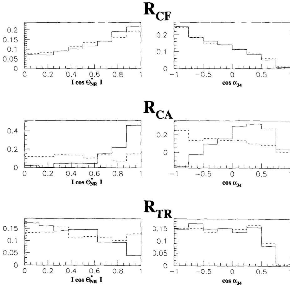
Fig. 6. Comparison of the shapes of the projections on the  $|\cos \theta_{NR}^*|$  and  $\cos \alpha_{34}$  axes of the two-dimensional distributions used in the fit. The full lines show the shapes of the distributions of correctly  $b$ -tagged events, the dashed lines show those of the events in which the jets are assigned incorrectly.
