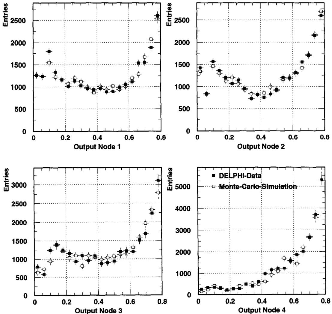
Fig. 4. Output of the four different nodes of the neural network using DELPHI data (filled boxes) and simulation (open boxes). Nodes 1–4 correspond to jets 1–4 numbered in order of decreasing energy. All of the distributions have high peaks for outputs above 0.8 (not shown). A jet with output below 0.5 was classified as a quark jet. Only events with exactly two jets classified as quark jets were used in the analysis.
