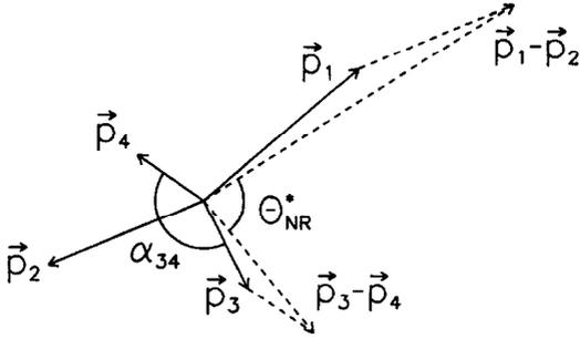
Fig. 2. Definitions of the generalised Nachtmann-Reiter angle  $\theta_{NR}^*$  and of the angle  $\alpha_{34}$ , which are the two angles used in the analysis:  $\vec{p}_1$  and  $\vec{p}_2$  are the momentum vectors of the two primary jets,  $\vec{p}_3$  and  $\vec{p}_4$  are those of the secondary jets,  $\theta_{NR}^*$  is the angle between  $\vec{p}_1 - \vec{p}_2$  and  $\vec{p}_3 - \vec{p}_4$ , while  $\alpha_{34}$  is the angle between  $\vec{p}_3$  and  $\vec{p}_4$ .
