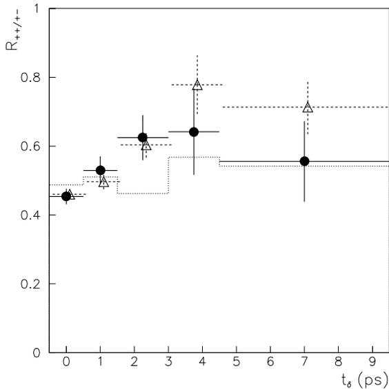
**Fig. 1.** Ratio  $R_{++/+-}$  of the  $t_{\delta}$  distributions obtained from same sign and opposite sign dilepton events when both leptons have a  $p_t$  greater than 1 GeV/c. Black circles correspond to real data events, triangles to simulated events with  $\Delta m = 0.47 \text{ ps}^{-1}$ . The dotted histogram corresponds to the hypothesis of time independent mixing
