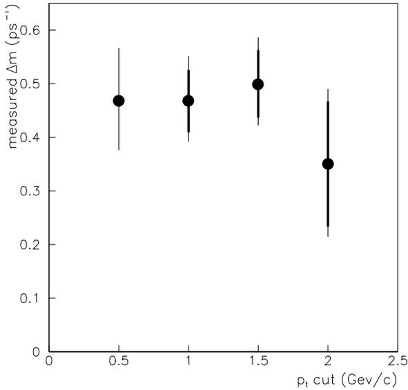
**Fig. 3.**  $\Delta m_d$  values measured for different  $p_t$  cuts. The thin error bars show the total statistical errors. The thick error bars show the error on the difference between the given point and the adjacent one for a smaller  $p_t$  cut
