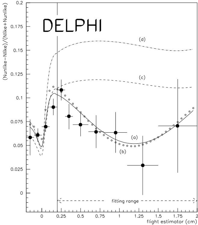
**Fig. 9.** Ratio  $(N_{unlike\ sign} - N_{like\ sign}) / (N_{unlike\ sign} + N_{like\ sign})$  as a function of  $\lambda$ . The curves are the expected shapes for (a) the fitted time-dependent oscillation (full curve), (b) the same without smearing the values of  $\lambda$  (open circles), (c) a time-independent mixing with  $\chi_d = 0.17$  (dashed curve), and (d) no mixing (dot-dashed curve)
