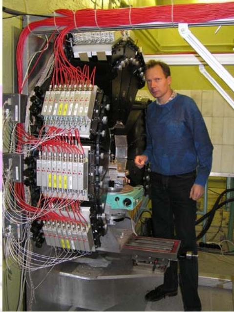
Epsilon-MDS and SKAT diffractometers complex for studies of geological materials
