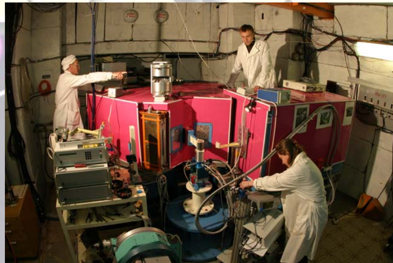
HRFD – high resolution Fourier diffractometer
