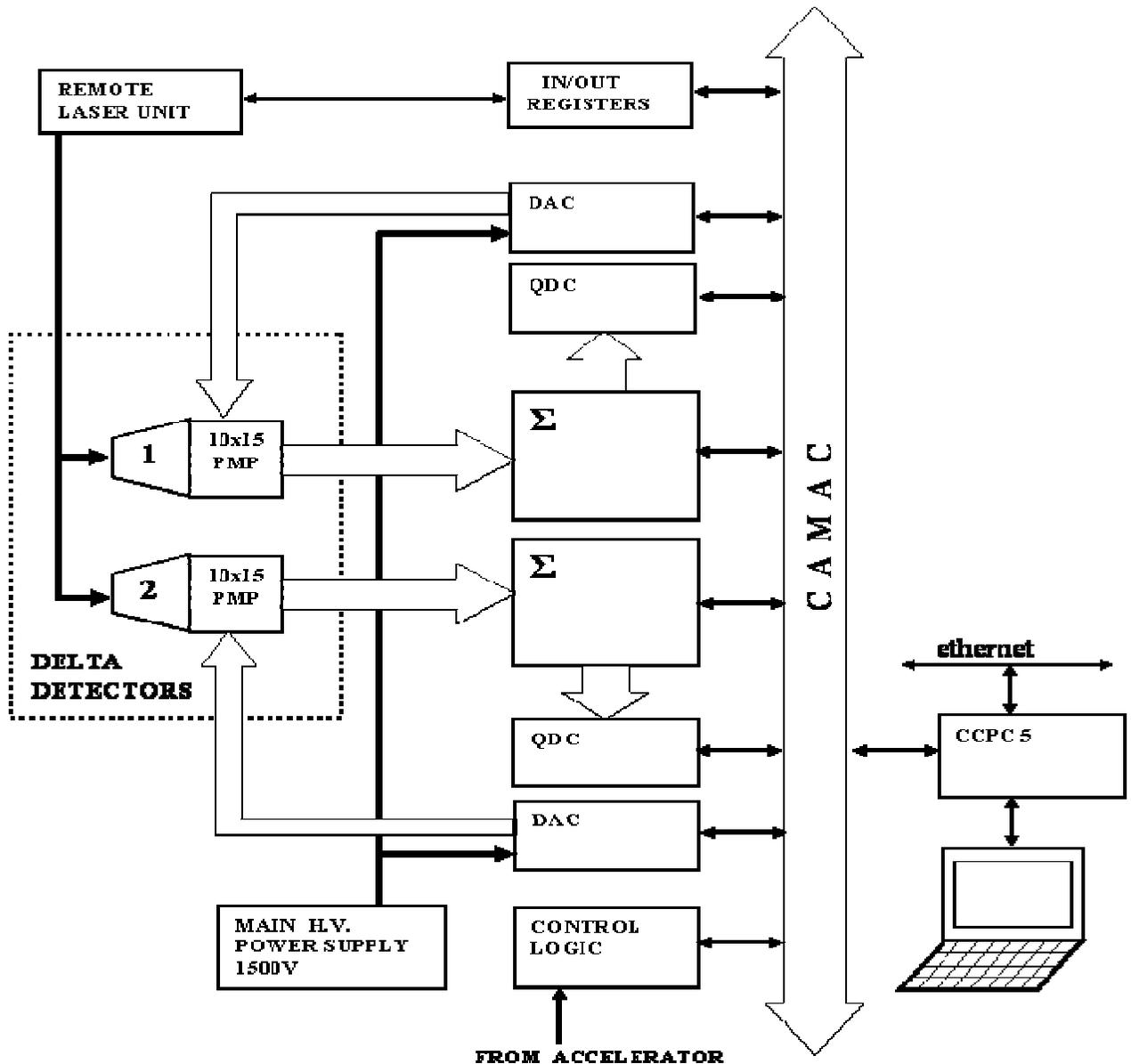
The data acquisition is organized by the intelligent CAMAC crate controller of type CCPC5 containing PC compatible computer. The whole data acquisition system consists of 4 CAMAC crates (EUR4100) organized in a branch. The crate 0 is controlled by the CCPC5 and contains branch driver. The other crates are connected via standard branch (EUR 4600) using the crate controller of type A1. The functional user modules placed in crates are described in brief in Appendices.
