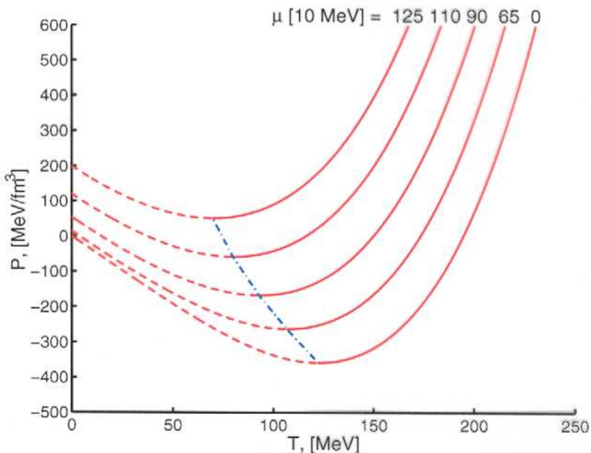
QGP EoS, with temperature dependent Bag constant, is shown for different value of  $\mu$  - full + dashed line. The spinodal is shown by dot-dashed line
