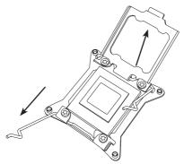
2. Use your thumb and index finger to hold the CPU on its edges. Align the CPU keys, which are semi-circle cutouts, against the socket keys.
