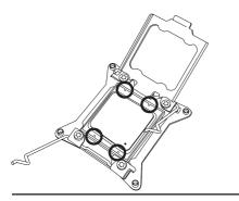
Warning: You can only install the CPU inside the socket in one direction. Make sure that it is properly inserted into the CPU socket before closing the load plate. If it doesn't close properly, do not force it as it may damage your CPU. Instead, open the load plate again and double-check that the CPU is aligned properly.
