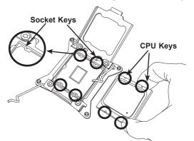
Once they are aligned, carefully lower the CPU straight down into the socket. (Do not drop the CPU on the socket. Do not move the CPU horizontally or vertically. Do not rub the CPU against the surface or against any pins of the socket to avoid damaging the CPU or the socket.)
