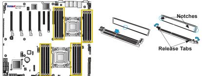
Align the key of the DIMM module with the receptive point on the memory slot.
