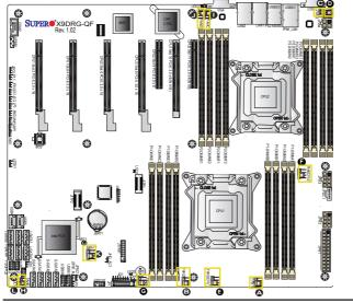
A. Fan 1 B. Fan 2 C. Fan 3 D. Fan 4 E. Fan 5 (CPU1 Fan) F. Fan 6 (CPU2 Fan) G. Fan A H. Fan B I. Fan C J. Fan D K. Fan 11 L. Chassis Intrusion
