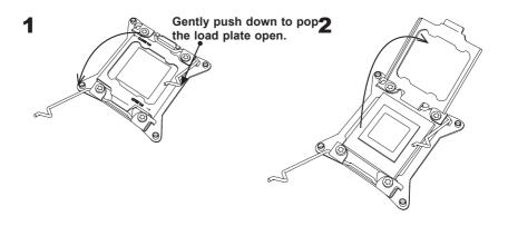
1. Use your index fingers to loosen the lever and open the load plate.
