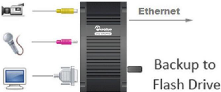
Figure 46 A USB Flash Drive Connected to a USB port Receives Recorded Data
