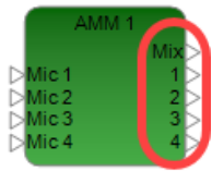
AMM Gain-Sharing Block - Standard with mix and direct outputs
