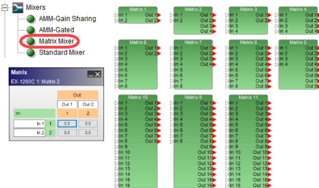
Matrix Mixer processing blocks and 2x2 control panel
