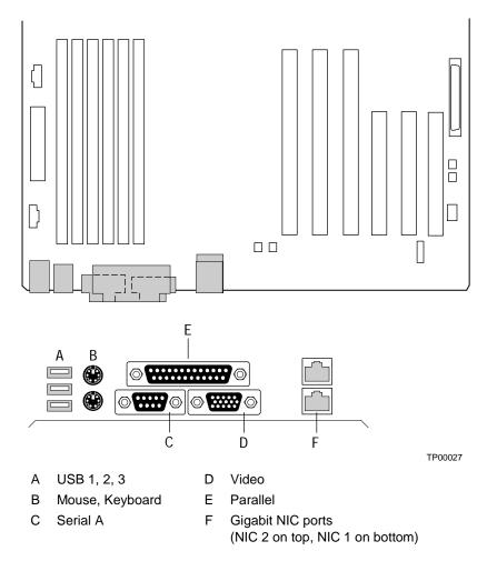
Figure 2. Back Panel Connectors
