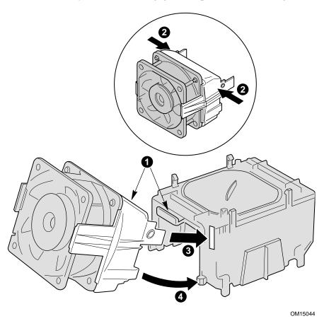
Figure 14. Attaching the Heat Sink Fan to the Top of the PWT
