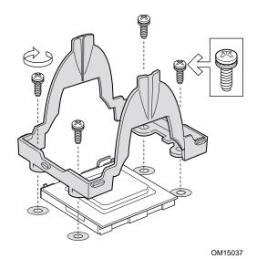
Figure 10. Attaching Retention Mechanism
