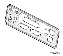
Figure 4. Attaching the Label to the I/O Shield
