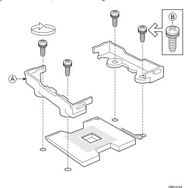
Figure 17. Installing the Processor Retention Brackets
