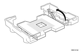
Figure 18. Raising the Locking Bar
