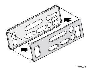
Figure 3. Attaching the Gasket to the I/O Shield
