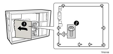
Figure 8. Placing the Server Board in the Chassis
