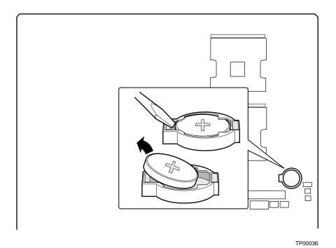
Figure 31. Replacing the Back up Battery
