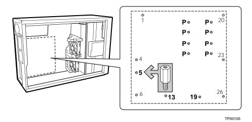
Figure 6. Installing Chassis Standoffs
