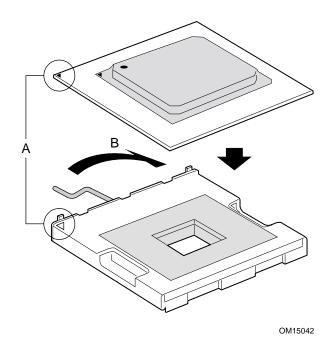
Figure 9. Opening Socket Lever and Attaching Processor
