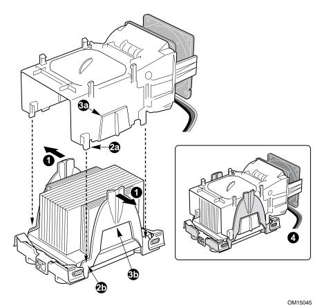
Figure 15. Attaching the Top Assembly to the Retention Mechanism
