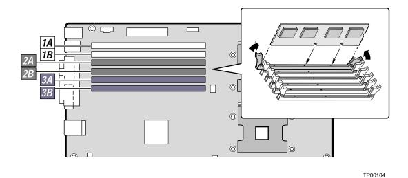
Figure 24. Installing Memory
