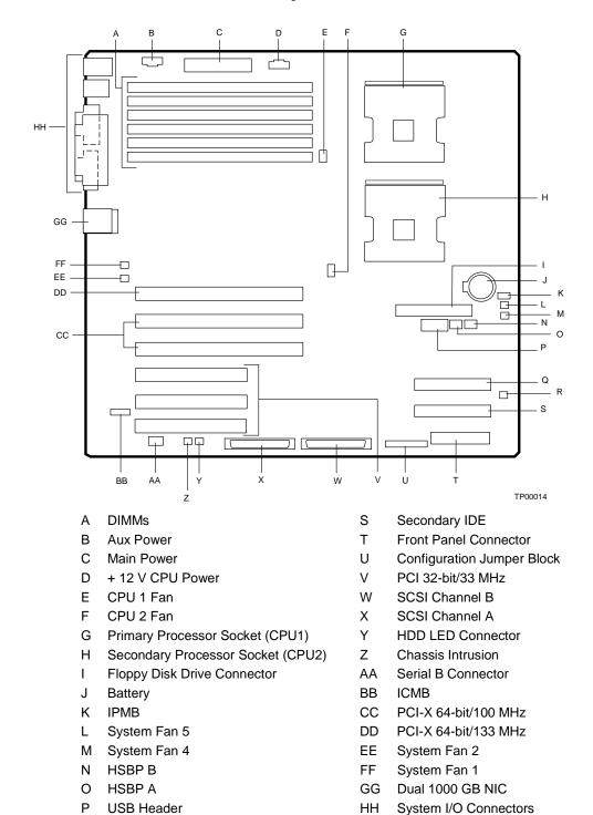
Figure 1. Server Board Connector and Component Locations
