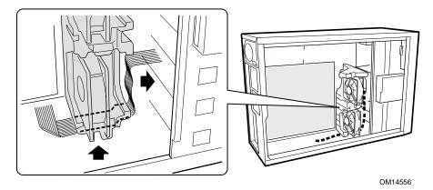
Figure 25. Routing Cables
