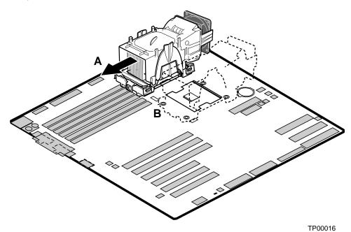
Figure 16. Processor and Wind Tunnel Installed
