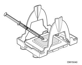
Figure 11. Applying Thermal Grease
