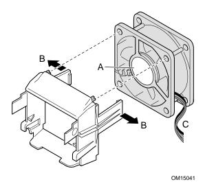
Figure 13. Attaching the Wind Tunnel Fan
