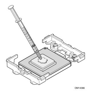
Figure 21. Applying Thermal Grease
