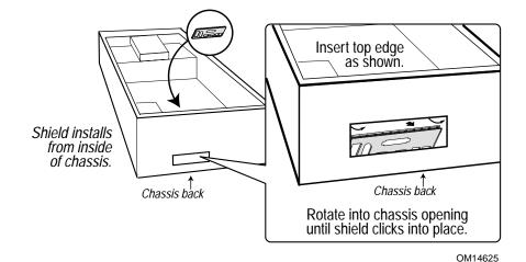
Figure 5. Installing the I/O Shield
