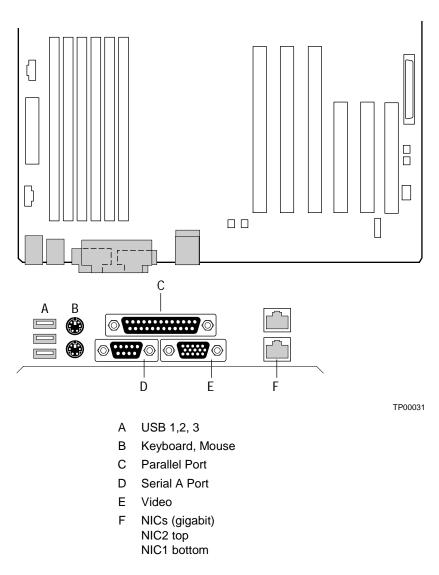
Figure 30. Making Back Panel Connections
