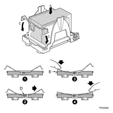
Figure 12. Attaching the Heat Sink and Retention Clip
