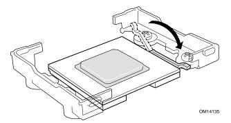
Figure 20. Lower Locking Bar
