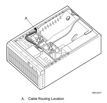
Figure 27. Routing the Floppy and ICMB Cables
