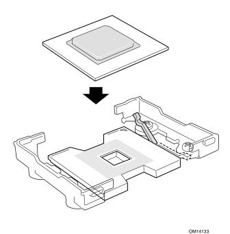
Figure 19. Installing Processors
