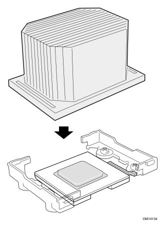
Figure 22. Installing the Heat Sink
