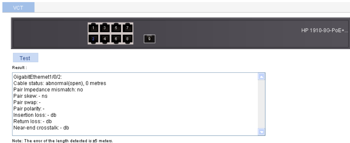
Figure 78 Testing the status of the cable connected to an Ethernet port
