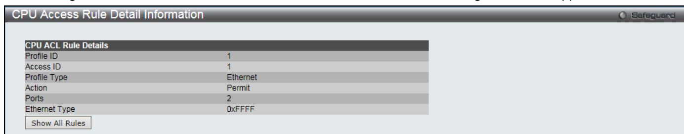
Figure 7-28 CPU Access Rule Detail Information (Ethernet ACL)
