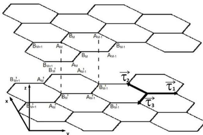
Fig. 1. Structure of finite-width graphene bilayer.
