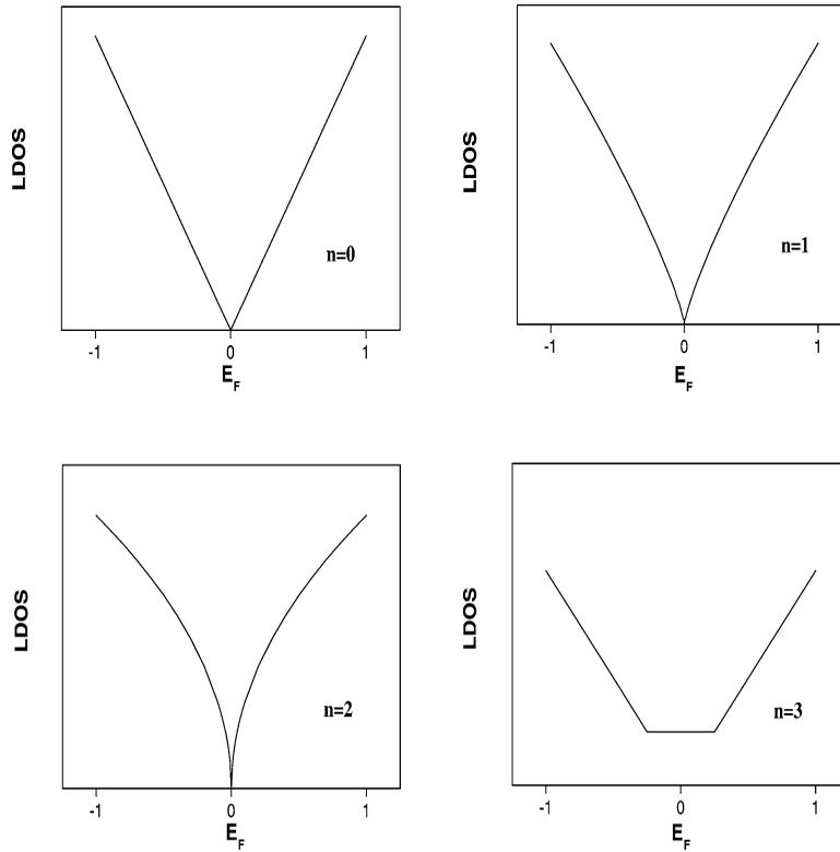
Fig. 2. Schematic densities of states near the Fermi energy in the case of cone.
