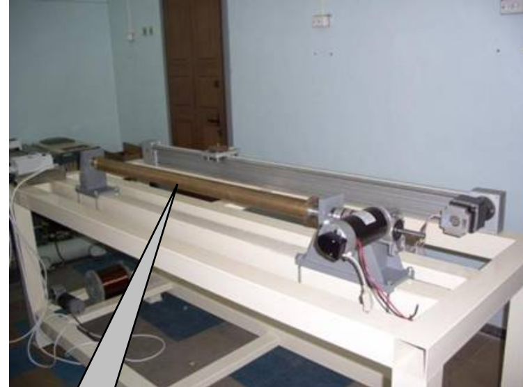
Automated tool for solenoid spooling
