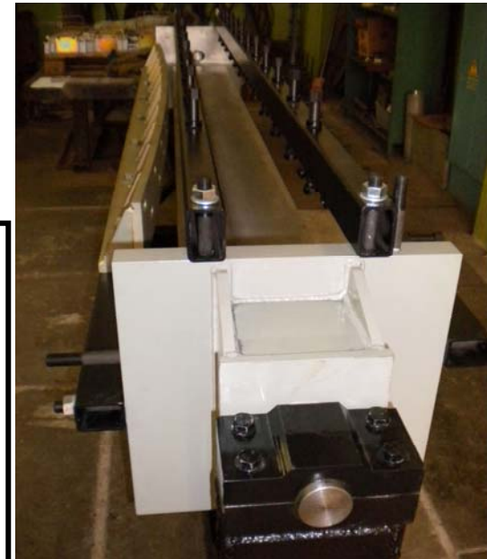
The tool for assembling a curved yoke for the Booster dipoles
