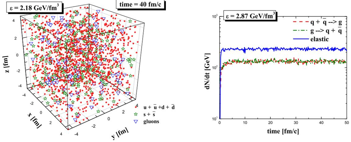
**Figure 1.** a) Snapshot of the spatial distribution of light quarks and antiquarks (circles), strange quarks and antiquarks (stars) and gluons (triangles) at a time of 40 fm/c. b) The reaction rates for elastic parton scattering (solid), gluon splitting (dash-dot) and flavor neutral  $q\bar{q}$  fusion (dash) as a function of time.
