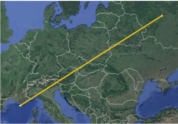
Fig. 3 Path to be traveled by the neutrino beam from Protvino (in the top right) to ORCA (in the bottom left). The path length is \approx 2595 km and the deepest point is 135 km below sea level, in the upper mantle
