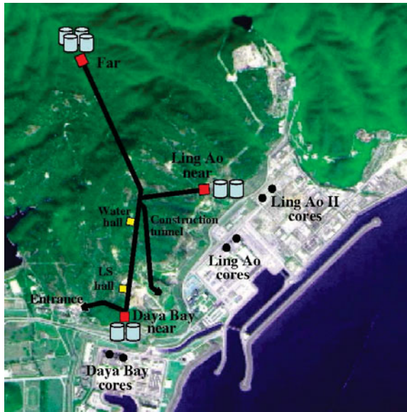
Fig. 5.5 The layout of the Day Bay reactor antineutrino experiment. Two pairs of reactor cores (Daya Bay and Ling Ao) are running and the third one (Ling Ao II) will run soon. Four detector modules are deployed at the far site, and two detector modules are deployed at each of the two near sites (Guo et al. , 2007)
