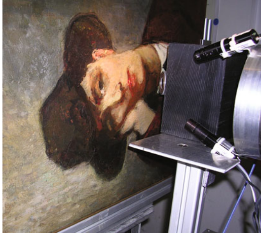
■ Fig. 9 Portrait attributed to Modigliani in the high-energy PIXE setup
