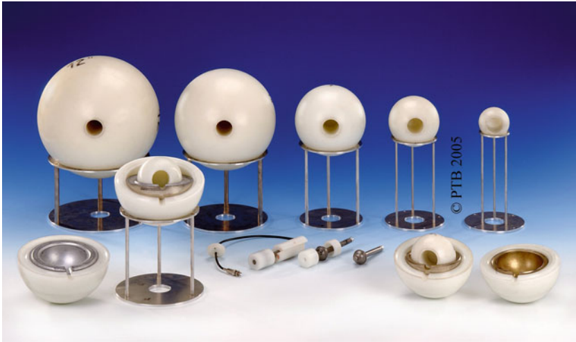
■ Fig. 5 Bonner sphere spectrometer NEMUS of the PTB with five of the ten polyethylene spheres in the back, a spherical ^3\text{He} proportional counter in the center, and parts of the modified spheres in the foreground left and right
