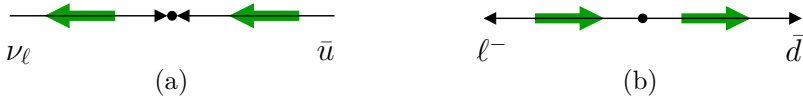
FIG. 5.13. (a) Configuration of the initial state in the process \nu_\ell + d \rightarrow \ell^- + u in the center-of-mass frame. The thin and thick arrows represent, respectively, momentum and spin. (b) Configuration of the final state in the same process with the charged lepton emitted backwards ( y = 1 ).
