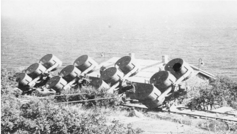
Fig. 6.11 Photograph of the Crimean multi-telescope setup. Each barrel contains one Cherenkov telescope. Three telescopes form a unit. Each of those units can be positioned along a railway system and view the air showers under slightly different angles. This arrangement allowed both coincidence measurements and simple multi-telescope observations. The system was used from 1960 until 1963. Figure courtesy T.C. Weekes
