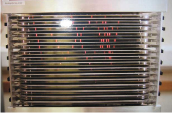
Fig. 4.18 The flash chamber built by the Laboratório de Instrumentação e Partículas (LIP) in Lisbon for didactical purposes records a shower of cosmic rays
