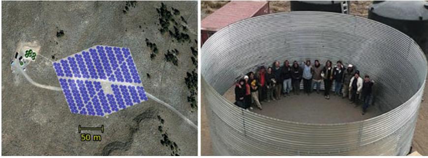
Fig. 4.50 Left Layout of the HAWC detector. The location of the different water tanks is shown. Right A water tank. Credit: HAWC Collaboration
