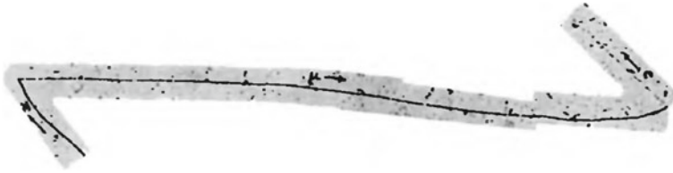
Fig. 3.11 The pion and the muon: the decay chain \pi \rightarrow \mu \rightarrow e . The pion travels from bottom to top on the left, the muon horizontally, and the electron from bottom to top on the right. The missing momentum is carried by neutrinos. From C.F. Powell, P.H. Fowler and D.H. Perkins, The Study of Elementary Particles by the Photographic Method (Pergamon Press 1959)
