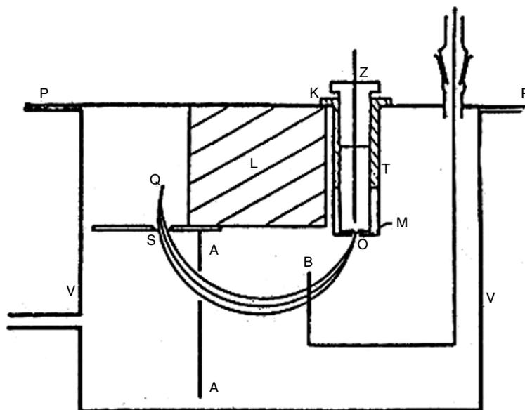
Fig. 1. The spectrometer used by Chadwick in the discovery of the continuous spectrum.
