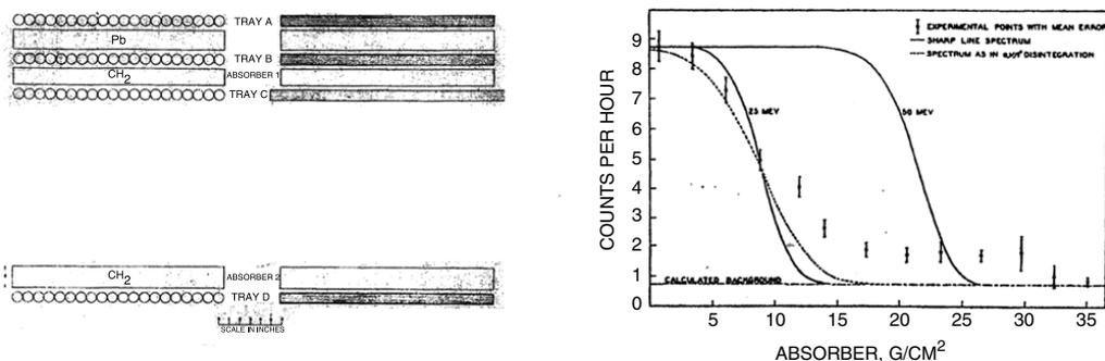
**Fig. 7.** My cosmic ray thesis experiment, measuring the electron spectrum in muon decay. Left: Detector with 80 Geiger counters. Right: The electron spectrum is continuous.
