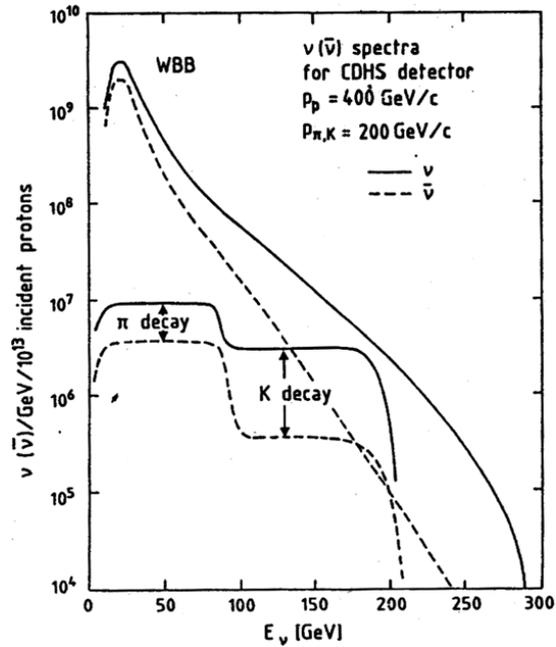
Fig. 25. Neutrino and antineutrino beam energy spectra. The lower flat spectra are the narrow band beams.
