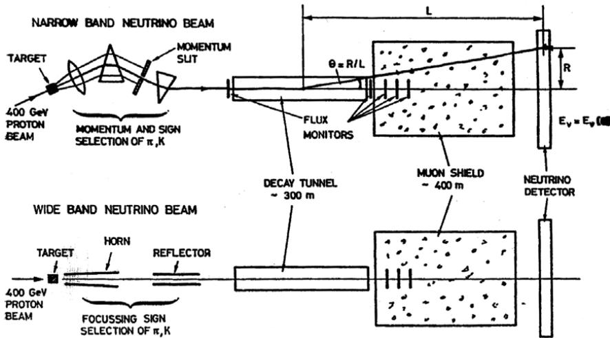
**Fig. 24.** Beam layouts at SPS.
