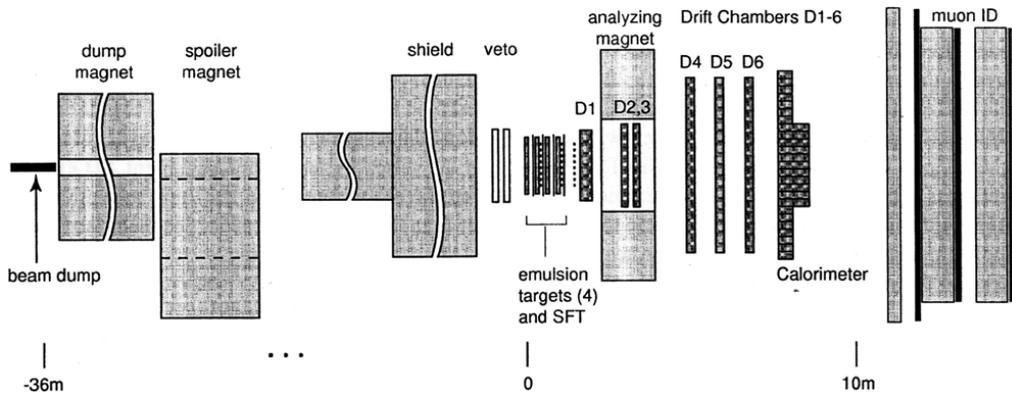
**Fig. 39.** Layout of DONUT experiment to detect tau neutrinos. SFT = Silicon Fiber Trackers.
