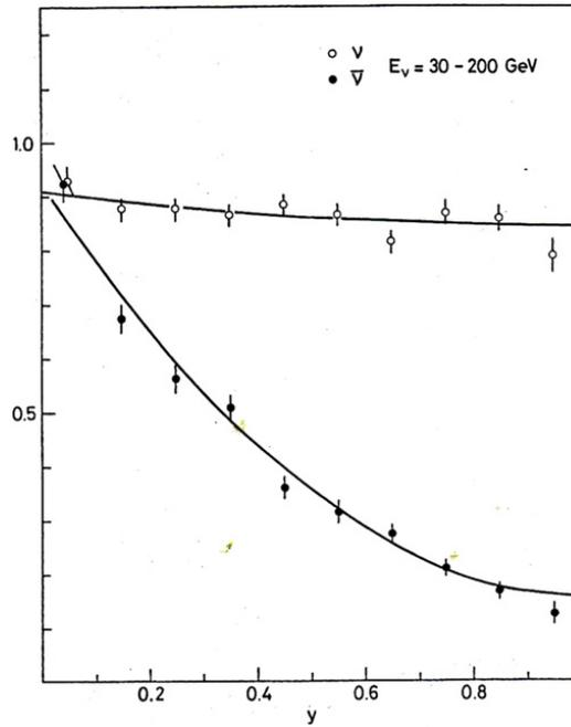
Fig. 31. CDHS results for the  $y$  distributions for neutrino and antineutrino cross-sections [24], in agreement with prediction of the parton model.
