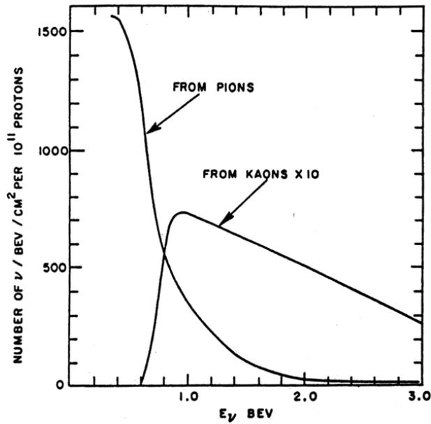
Fig. 13. Calculated energy spectrum of neutrino beam, pion and kaon contributions.
