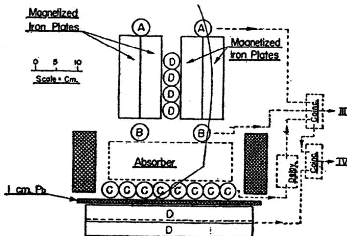
**Fig. 6.** The cosmic ray detector of Conversi et al.. The iron slabs above the detector were magnetized to focus either positive or negative muons. The decay electrons or positrons below the absorber plates were then detected.
