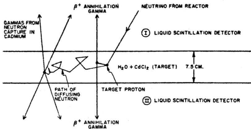
**Fig. 9.** Schematic diagram of the Reines and Cowan neutrino detector.
