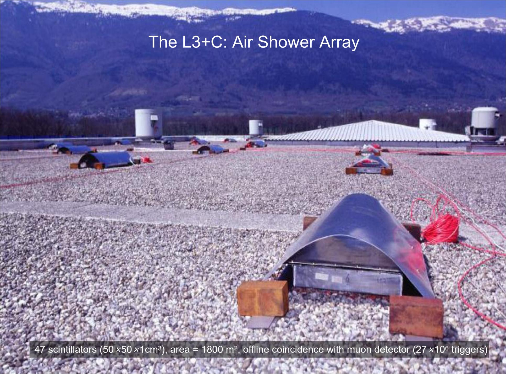
47 scintillators ( $50 \times 50 \times 1 \text{ cm}^3$ ), area =  $1800 \text{ m}^2$ , offline coincidence with muon detector ( $27 \times 10^6$  triggers)
