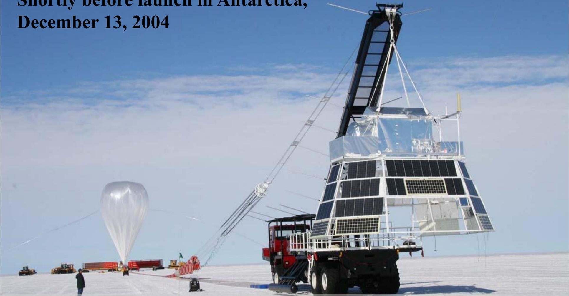
**BESS** (the **B**alloon-borne **E**xperiment with a **S**uperconducting **S**pectrometer) is a joint project of Japanese and US scientists to search for antimatter in the cosmic radiation, as well as measure energy and intensity of less exotic components of the cosmic radiation.
