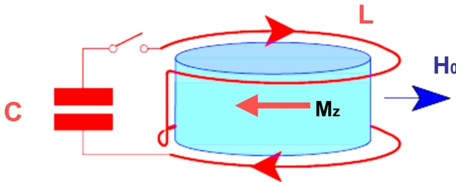
resonant circuit, tuned on the nuclear Larmor frequency, has no losses.
