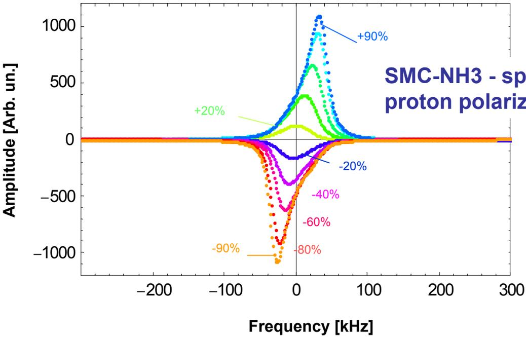
**SMC-NH<sub>3</sub> - spectra at different proton polarizations.**
