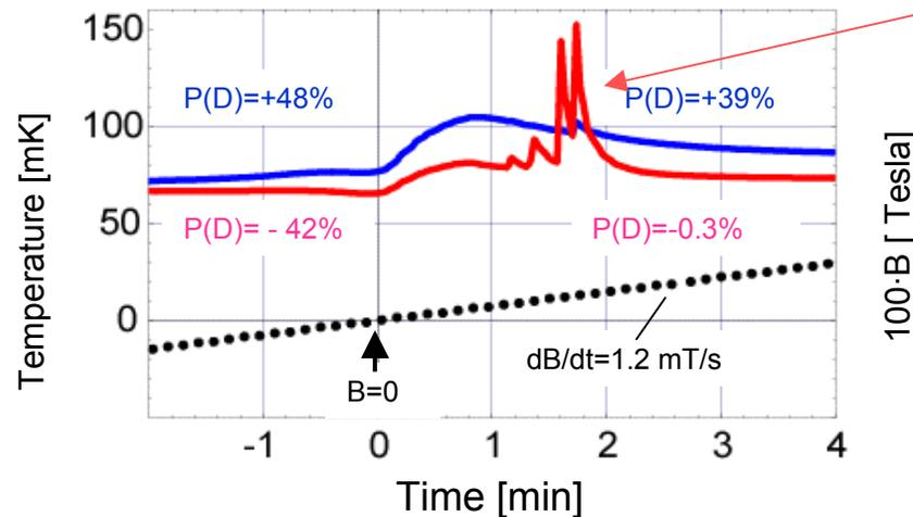
Here you can see the coherent radiation of D and Li7 obtained on the COMPASS polarized target at CERN
