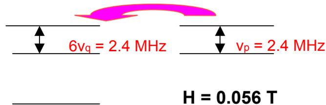
**N<sub>14</sub>-spins in NH<sub>3</sub> reach only 14% during usual DNP-polarization at 2.5 T and 0.1 K. But in 0.056 T field Zeeman proton and N<sub>14</sub> quadrupole energy splitting are equalized and for some millisecond interval polarized protons enlarged N<sub>14</sub> polarization up to 50 % .**
